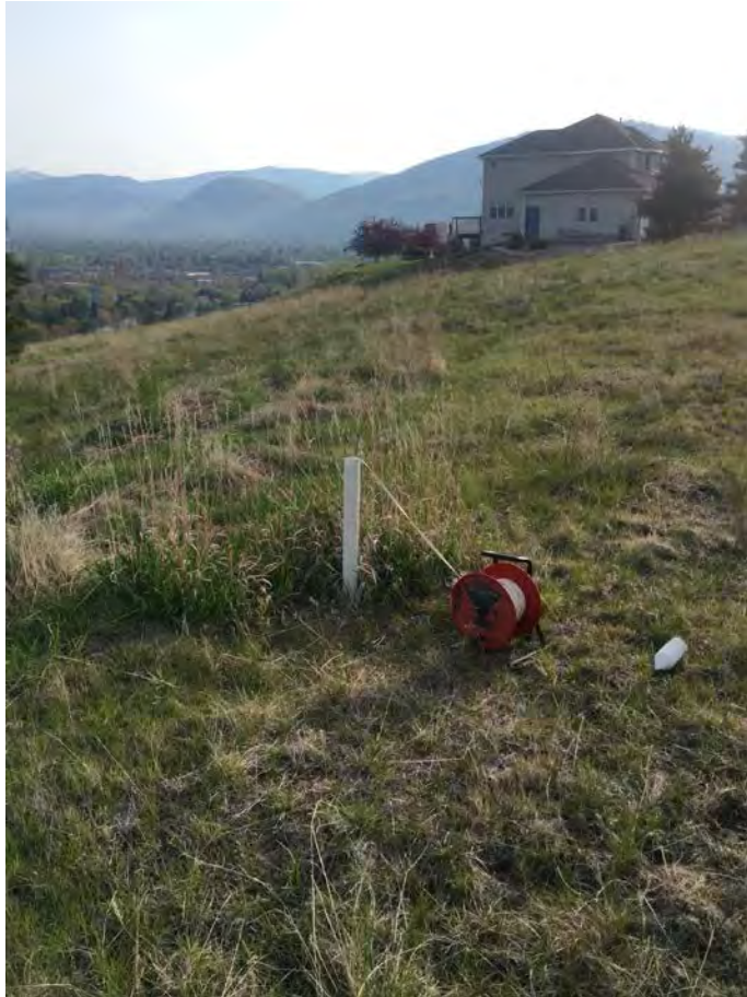
Piezometer ST-1P, groundwater at 42.7 feet
