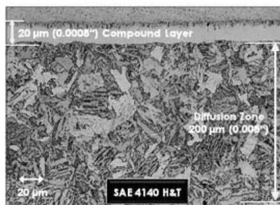
The **Compound Layer (CL)** is essentially  $\epsilon$  (epsilon) iron nitride + special nitrides (in case of alloyed steels) + some iron oxides.
