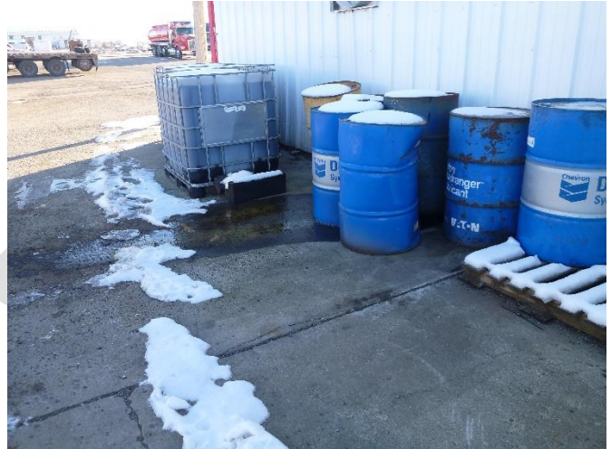
Uncontained and leaking waste oil at a truck maintenance facility being displaced by storm water to a nearby storm sewer.
