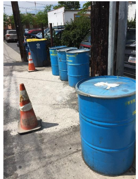
Cones were unable to prevent vehicle collisions and release of used cooking oil from these drums
