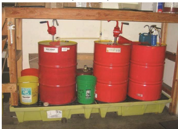
Prefabricated drum containment. Photo credit: Panhandle Health District
