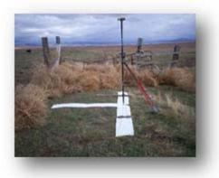
**Target Placement and Control Surveying.** Prior to photography, Morrison-Maierle will target and survey the 15 aerial control points shown in RED in the Exhibit B map. Control will tie to both Montana State Plane Coordinates. Horizontal datum shall be NAD 83 (2011); Vertical datum shall be NAVD 1988. Units shall be in US Survey Foot.
