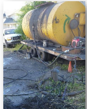
Improper maintenance of asphalt tank and insufficient SOPs for preventing ground contamination
