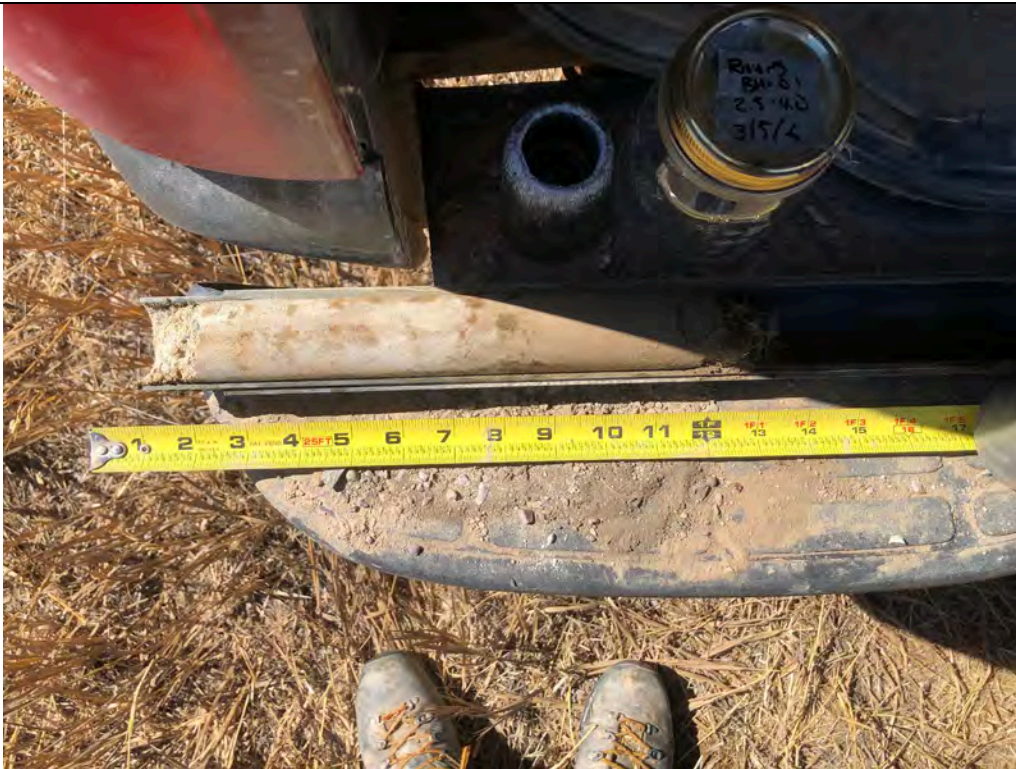
Description: BH-01 Split Spoon (SS) sample from the 2.5- to 4-foot depth.
