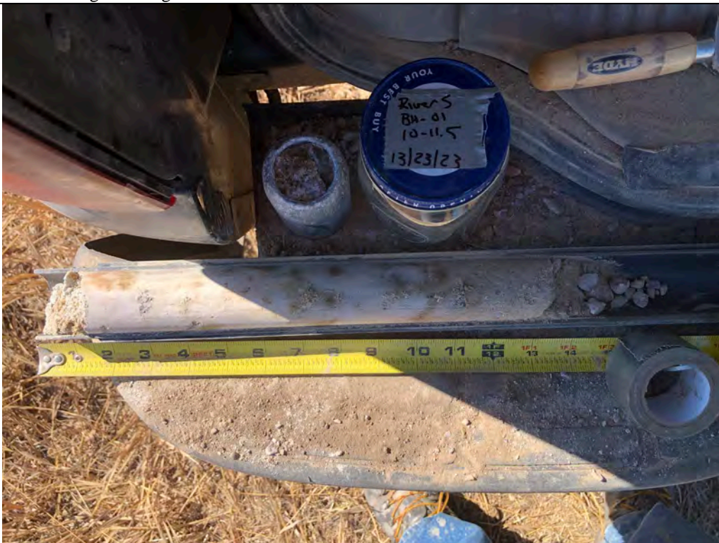
Description: BH-01 SS sample from the 10- to 11.5-foot depth.
