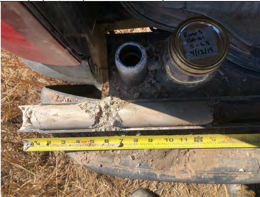
Description: BH-01 SS sample from the 5- to 6.5-foot depth.
