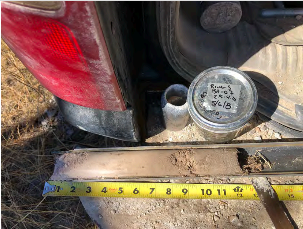
Description: BH-07 SS sample from the 2.5- to 4-foot depth.
