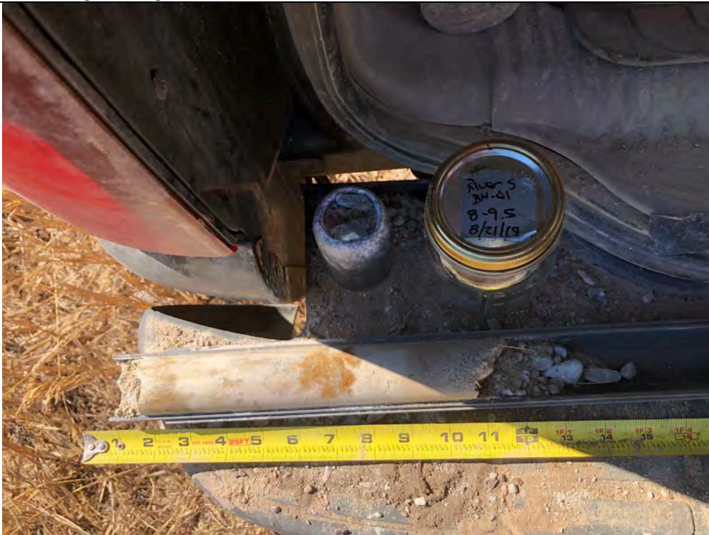
Description: BH-01 SS sample from the 8- to 9.5-foot depth.
