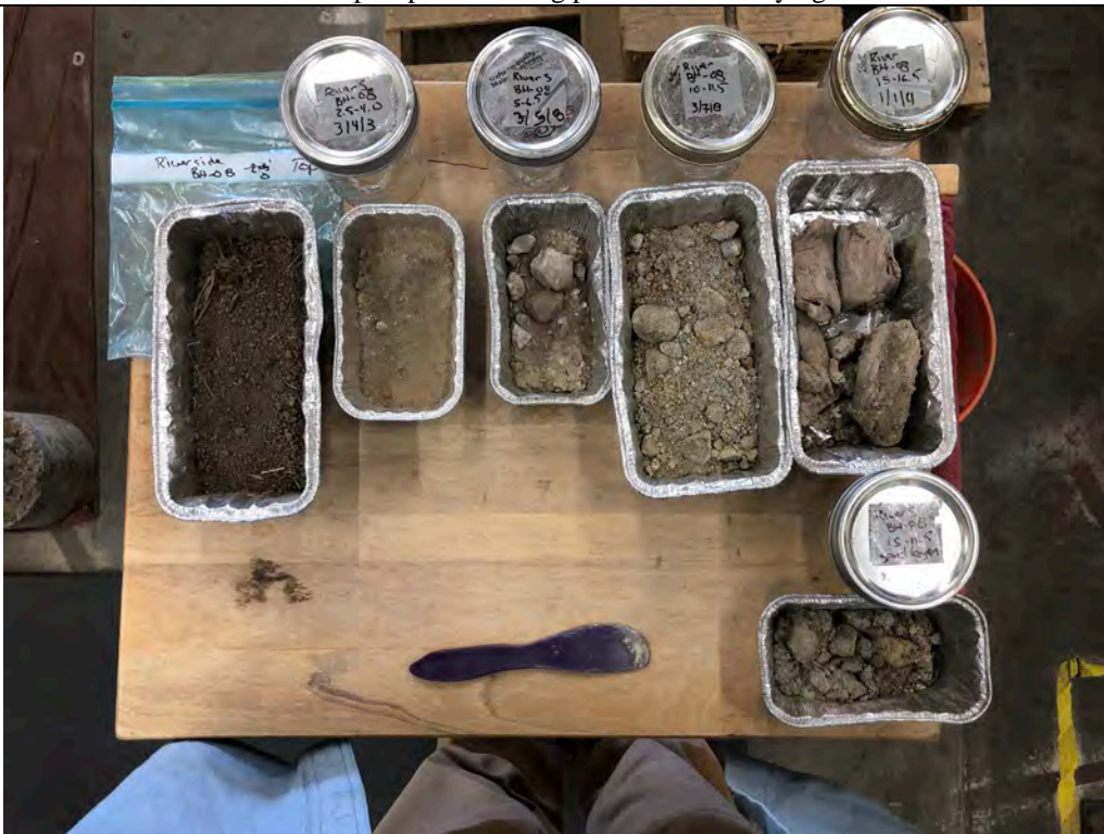
Description: BH-08 Moisture content samples after being taken out of the drying oven.
