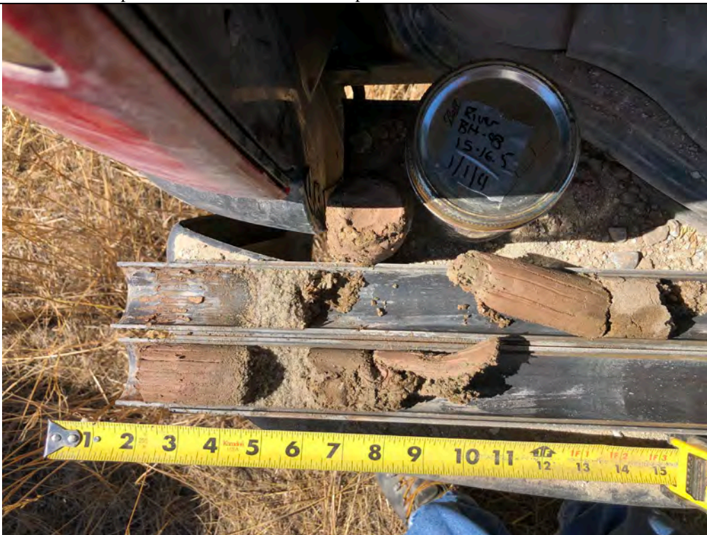
Description: BH-08 SS sample from the 15- to 16.5-foot depth.
