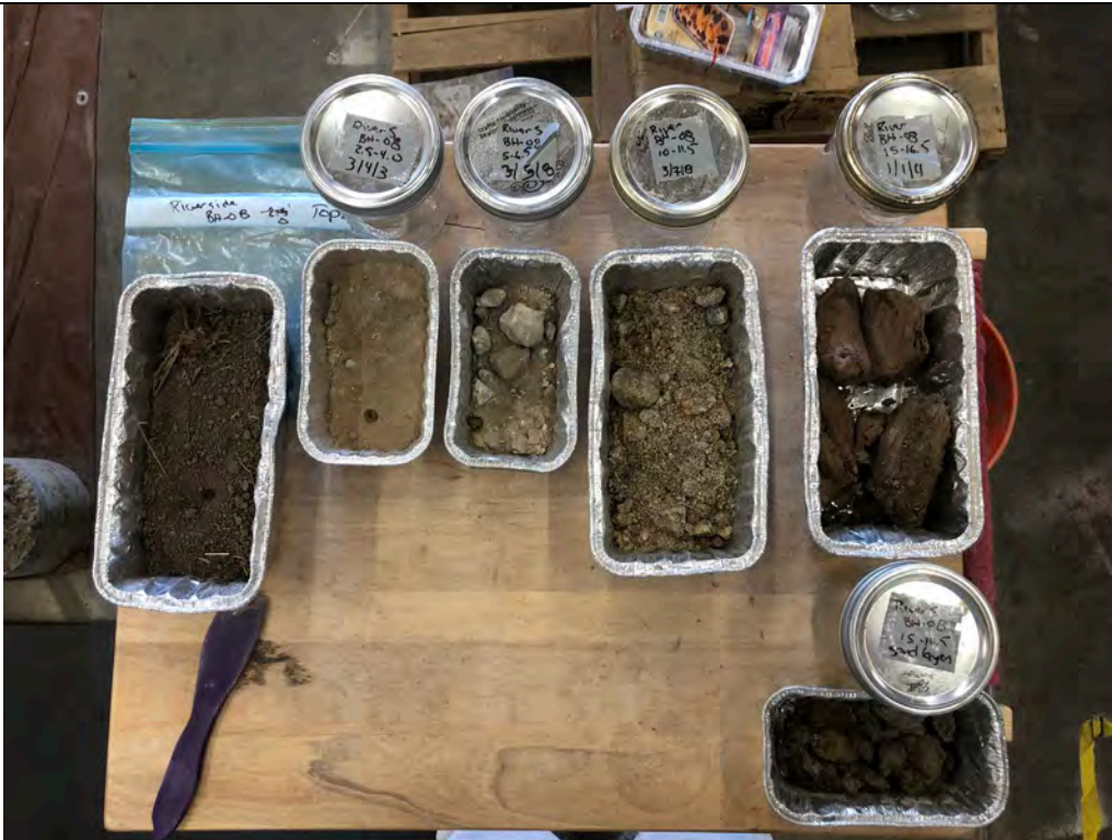
Description: BH-08 Moisture content samples prior to being placed into the drying oven.
