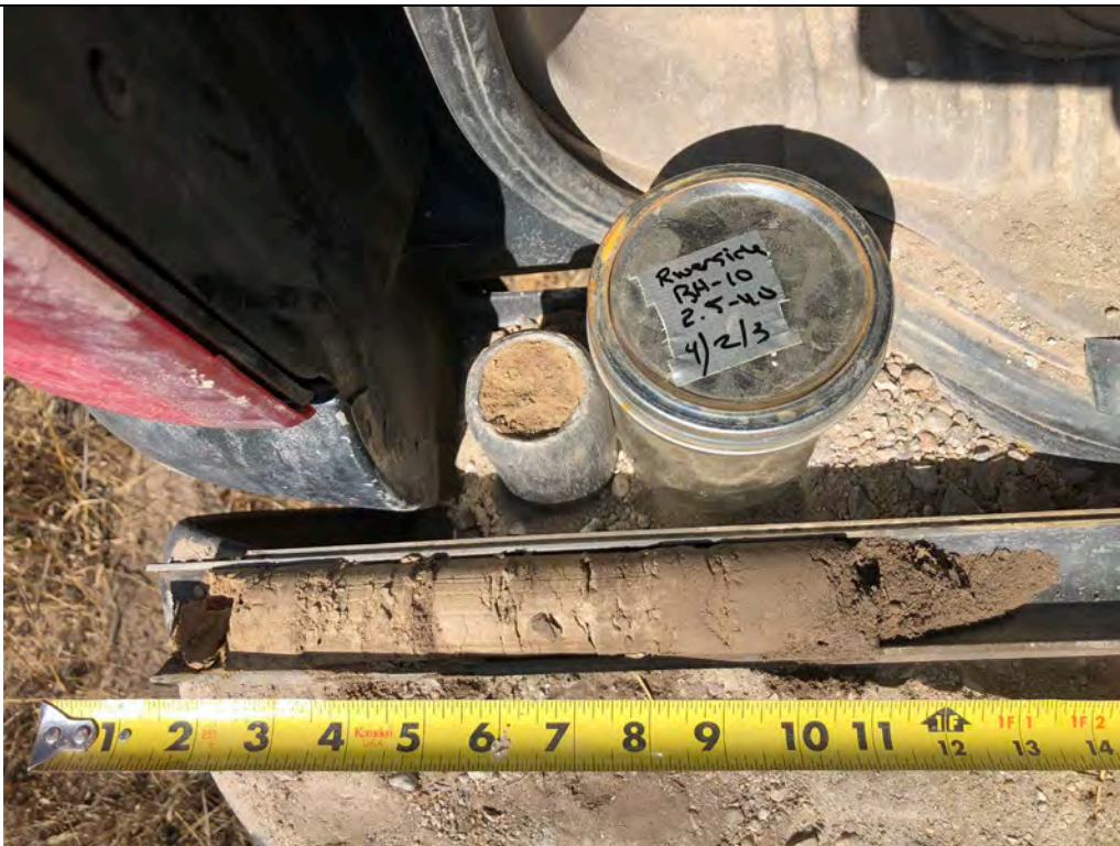
Description: BH-10 SS sample from the 2.5- to 4-foot depth.
