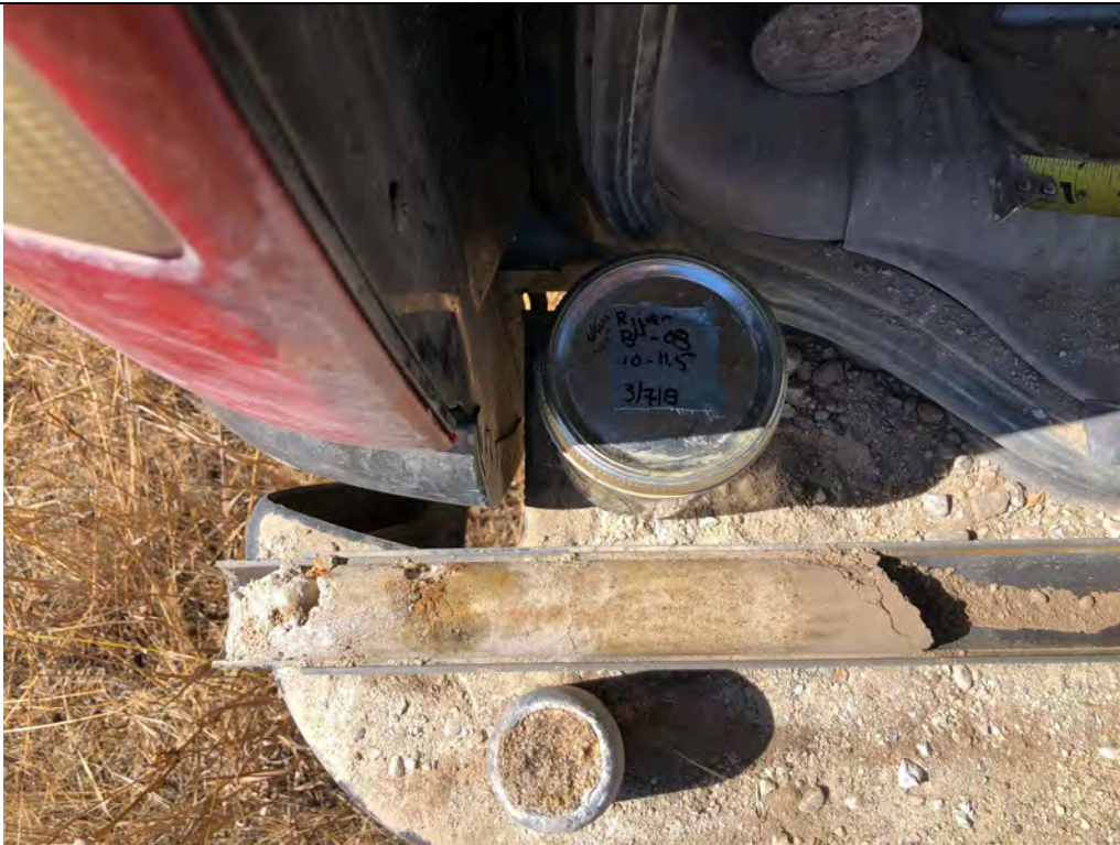
Description: BH-08 SS sample from the 10- to 11.5-foot depth.
