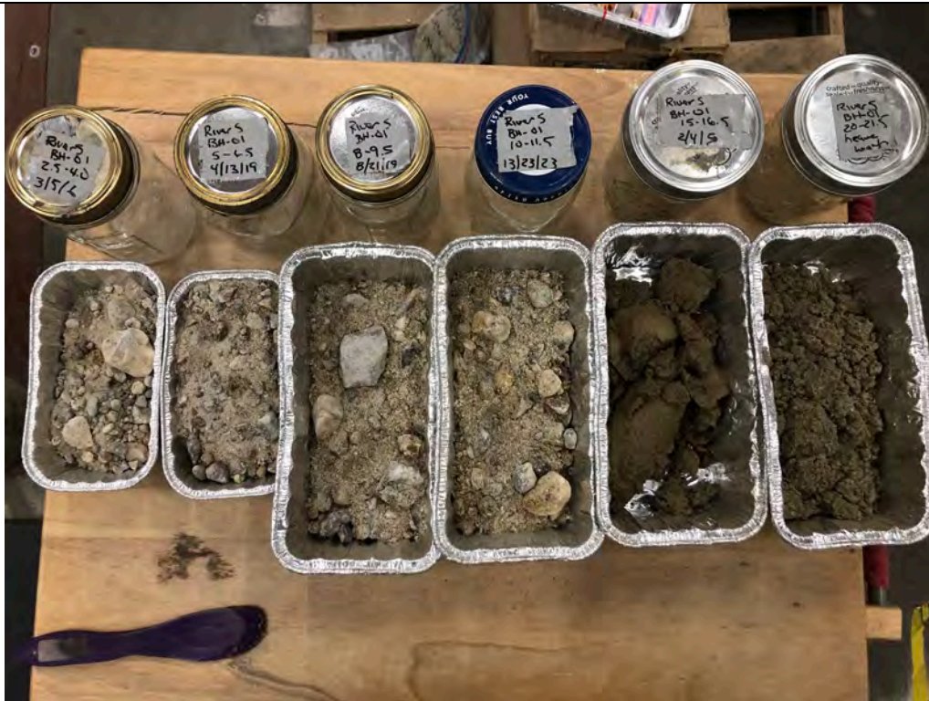
Description: BH-01 Moisture content samples prior to being placed into the drying oven.
