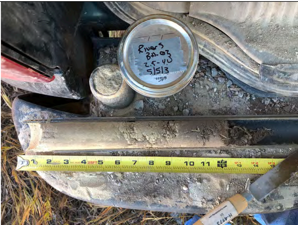
Description: BH-03 SS sample from the 2.5- to 4-foot depth.
