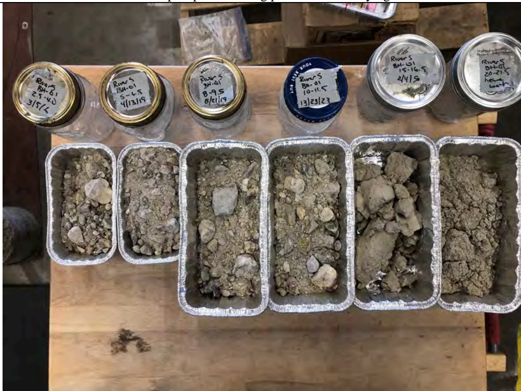
Description: BH-01 Moisture content samples after being taken out of the drying oven.
