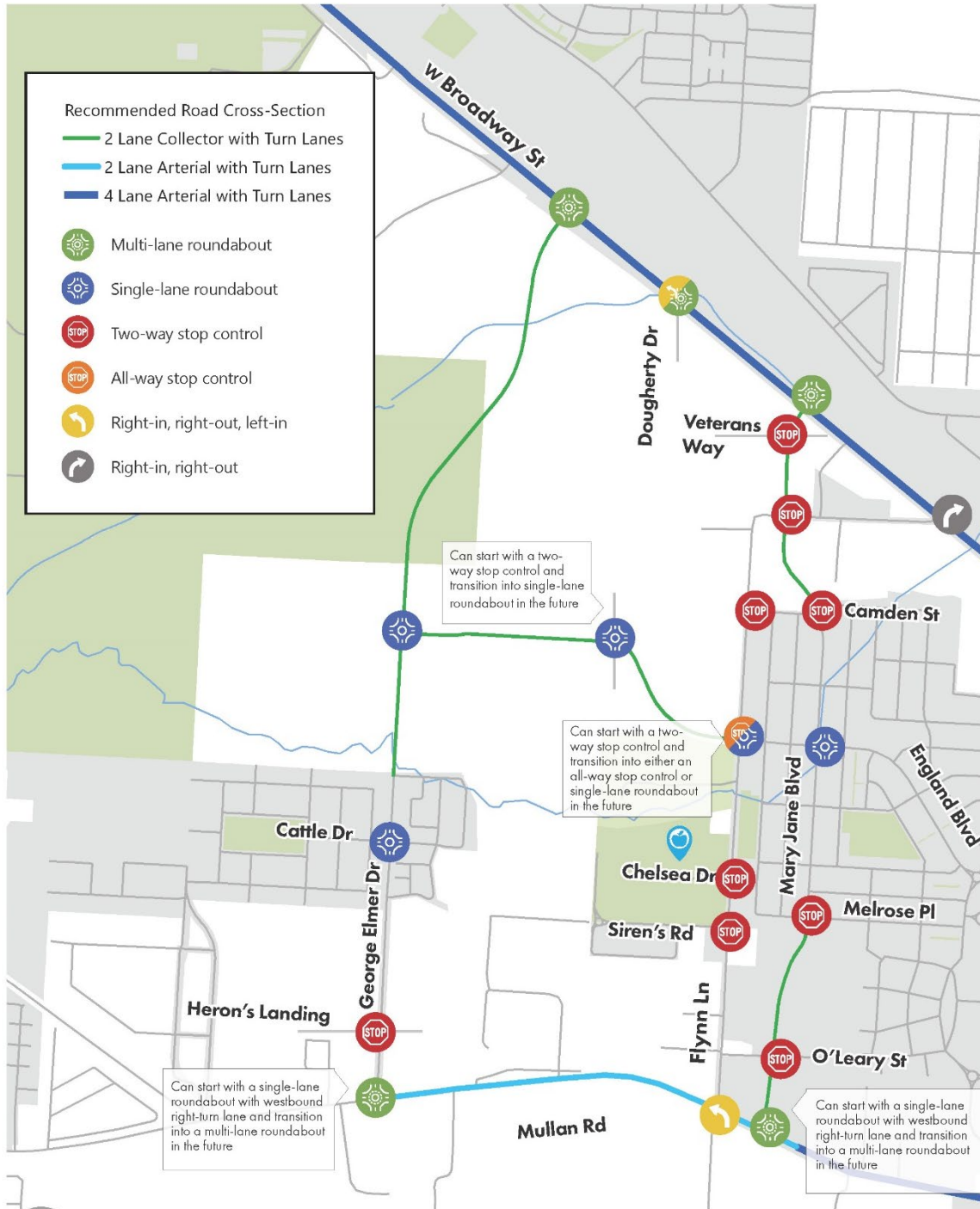
Figure 10 Intersection Control & Roadway Cross-Section Recommendations (2050)
