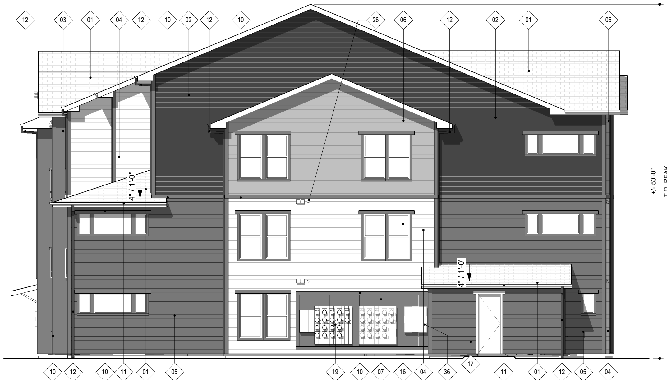
2 LEFT ELEVATION - BLDG TYPE B 1/8" = 1'-0"
