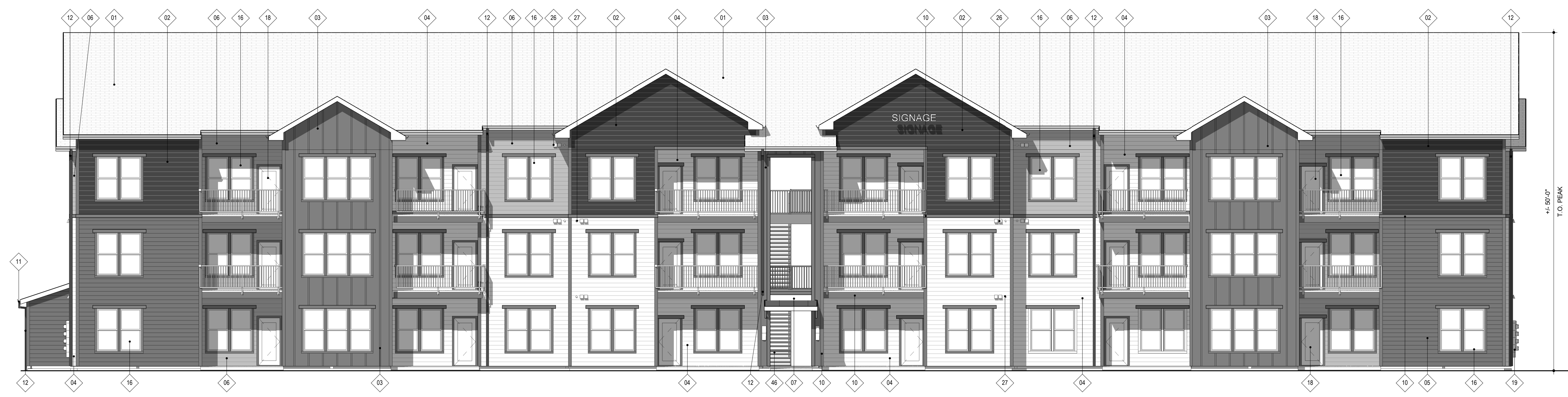
4 REAR ELEVATION - BLDG TYPE C 1/8" = 1'-0"
