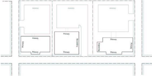
Figure 20.40-11 Primary and Secondary Facades
