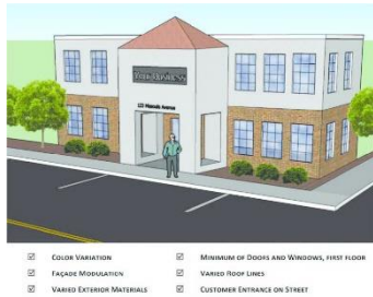
Figure 20.40-13 Building Incorporating All General Commercial Design Alternatives
