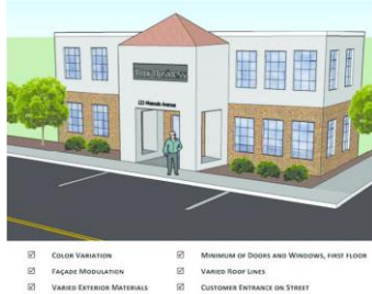
Figure 20.40-13 Building Incorporating All General Commercial Design Alternatives
