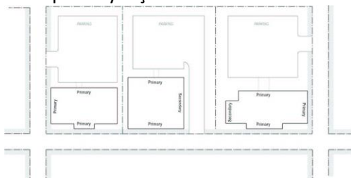
Figure 20.40-11 Primary and Secondary Facades
