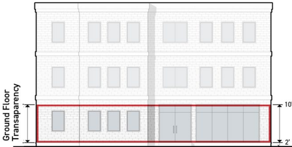
Figure 4.10.03-2 Ground Floor Transparency Measurement
