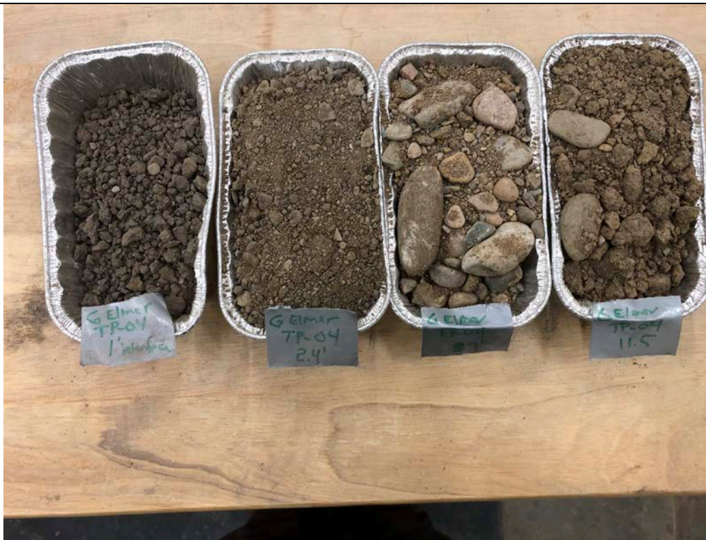
Description: TP-04 Moisture content samples after being taken out of the drying oven.
