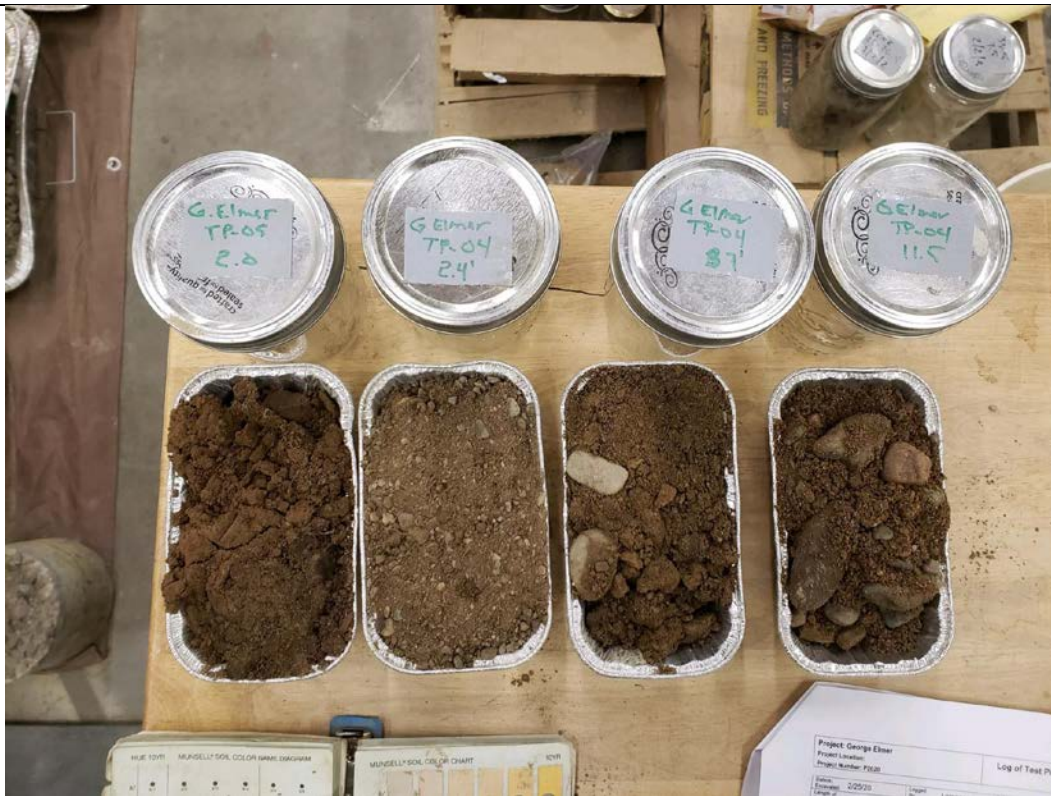
Description: TP-04 Moisture content samples prior to being placed into the drying oven. First jar should be with TP-05 photo.
