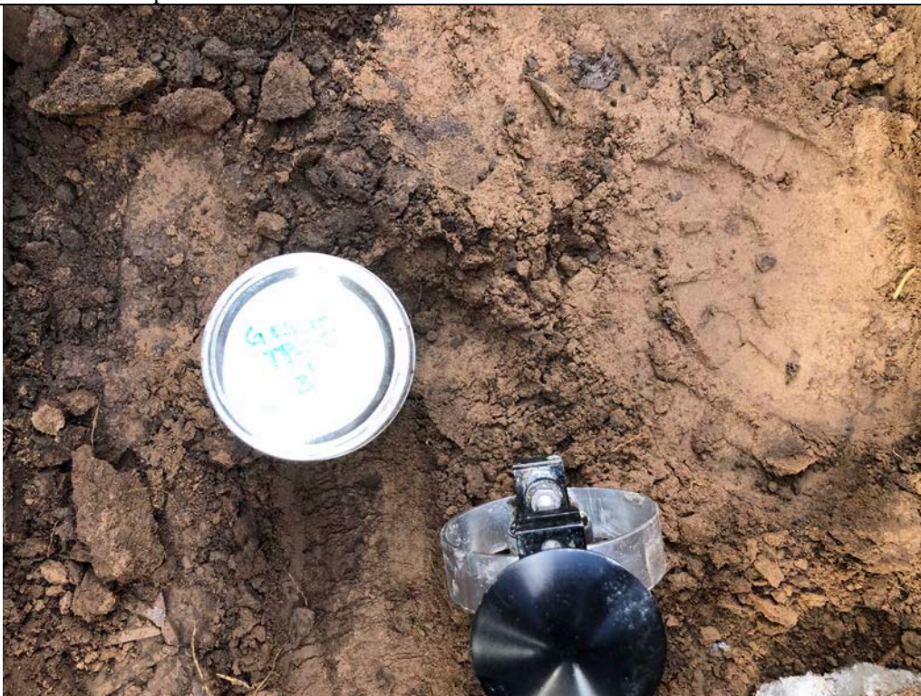
Description: TP-05 Jar sample from 3 feet. Cone penetrometer was pushed its full 21 inches under a 240 psi loading.
