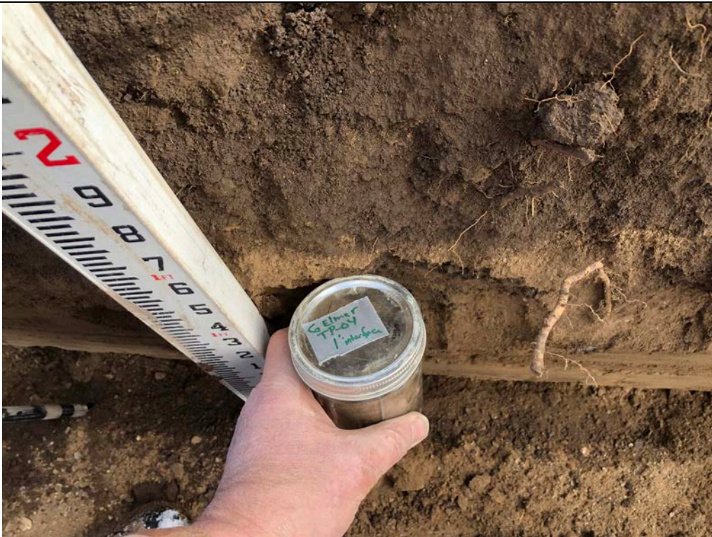
Description: TP-04 Jar sample from 1 foot. Below the color change interface. Test pit is excavated to 2.4 feet here.
