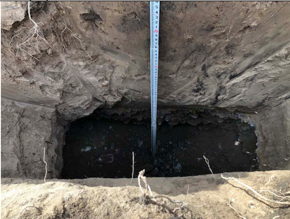
Description: TP-01 Excavated to 11.5 feet.
