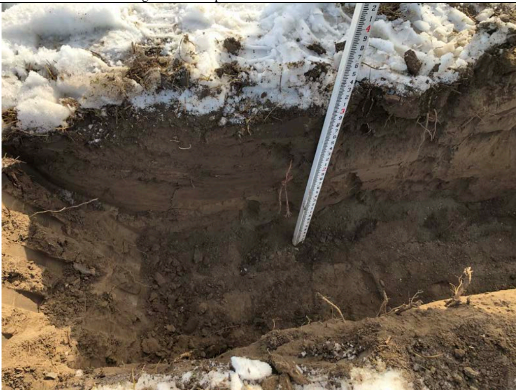
Description: TP-06 Plastic twine string at 1-foot depth.
