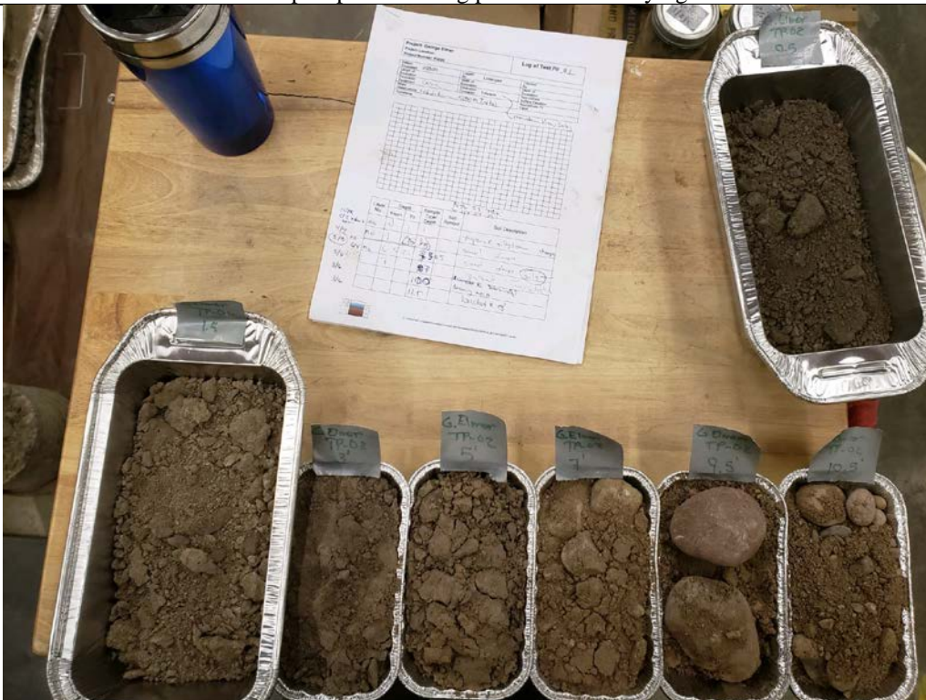
Description: TP-02 Moisture content samples after being taken out of the drying oven.
